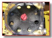
4 Remove the disc and fit the selected disc (the disc surface with the arrow should face you).
