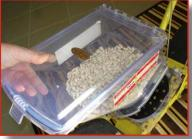
Remove the brush by pulling it upwards.
